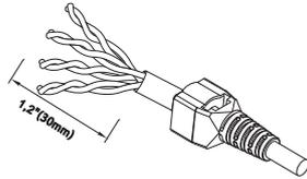
③ Fan out all four twisted pairs, following the color coding label and allocate each conductor into proper slots on wiring cap. Trim the ends of conductors.
