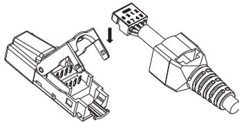
⑤ Place the wiring cap onto plug, use plier to clamp wiring cap until it completely snap-in to effect the connection.
